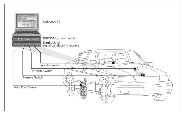
Riding in the passenger seat, researchers used the DaqBook to gather data from brake and accelerator pedals to monitor driver behavior (A & B), a sensor behind the driver's seat to measure vehicle swerving (C), and a non-contact wheel on the passenger door to log vehicle speeds and distances traveled (D).
